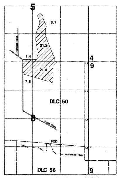
POD is located 200'S & 1630'E from NW corner of DLC 56.
