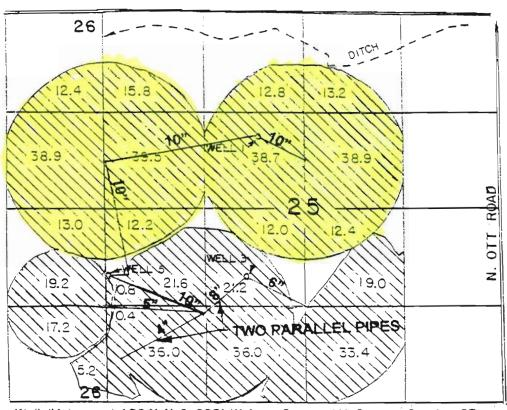
Well #1 located 1900' N & 600' W from Center 1/4 Corner, Section 25. Well #3 located 920' S & 760' W from Center 1/4 Corner, Section 25. Well #5 located 1750' N & 30' E from SW Corner, Section 25.
