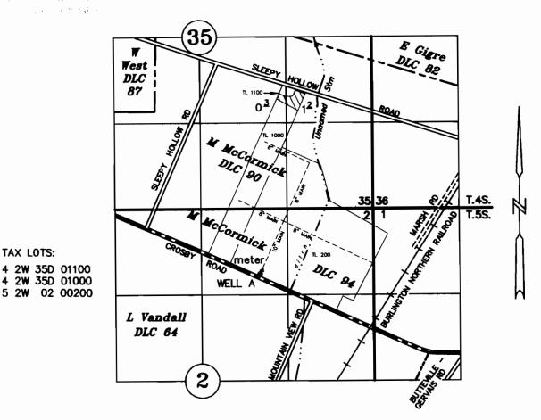
POA: 1190' NORTH & 2585' WEST OF NE COR. L. VANDALL DLC NO. 64 METER: 9' NORTH & 4' WEST OF WELL A (10' along pipeline)
