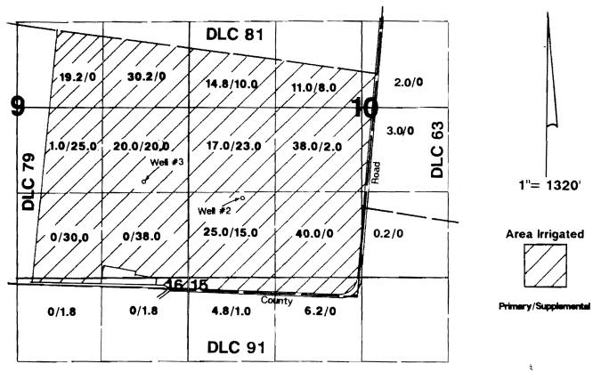
Well #2 located 1740'N & 1760'W from SE corner DLC 79. Well #3 located 1820'N & 3280'W from SE corner DLC 79.
