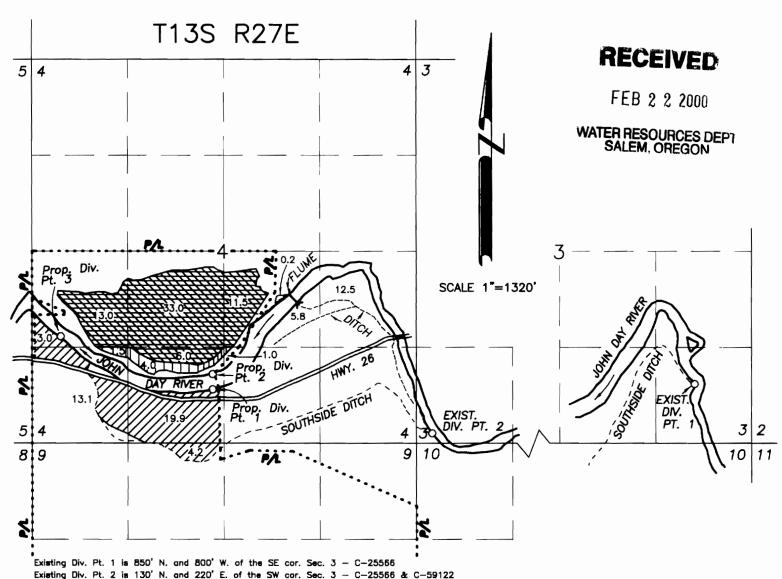
Existing Div. Pt. 2 is 130° N. and 220° E. of the SW cor. Sec. 3 — C Proposed Div. Pt. 1 is 700° N. and 2770° W. of the SE cor. Sec. 4. Proposed Div. Pt. 2 is 930° N. and 2800° W. of the SE cor. Sec. 4. Proposed Div. Pt. 3 is 1480° N. and 4860° W. of the SE cor. Sec. 4.
