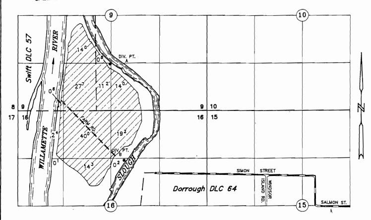
DIV. PT. A: 3110' NORTH AND 5695' WEST OF NE COR. DORROUGH DLC 64 DIV. PT. B: 437' NORTH AND 5304' WEST OF NE COR. DORROUGH DLC 64
