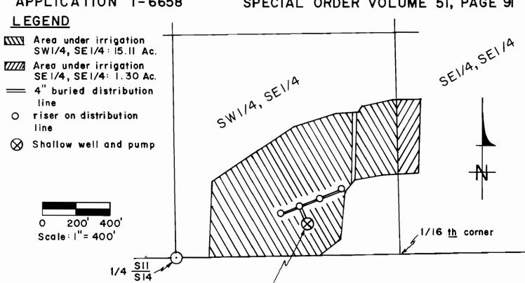
The pump and shallow well is located 185' North and 780' East of the 1/4 corner common to Section II and Section 14, T2N., R3IE., W.M.
