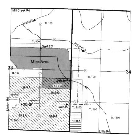
Well # 1 located 1150 ft N and 2050 ft W from SE corner of Section 33.
