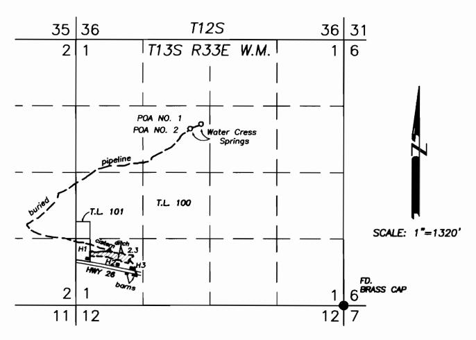
Point of Appropriation No. 1 is 3600' N. and 2830' W. of the SE Cor. Sec. 1. - 77420 Point of Appropriation No. 2 is 3510' N. and 3050' W. of the SE Cor. Sec. 1. - 77420
