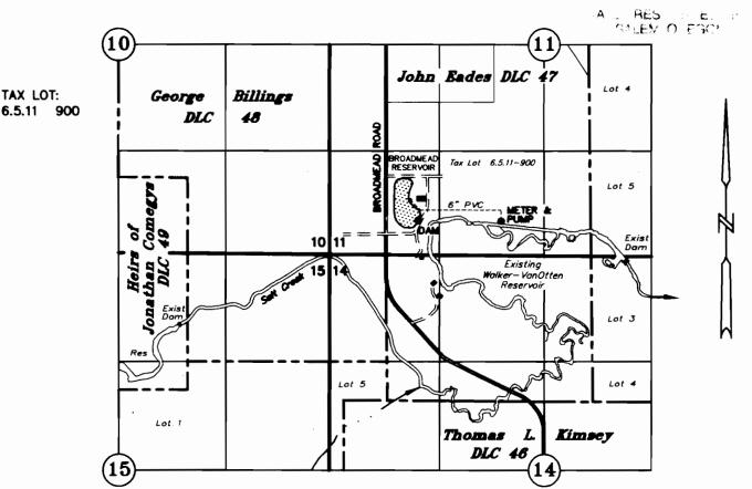
2228' North and 1405' East of the SW Corner John Eades DLC 47, POD 1: with approved fish screen on end of foot valve and meter at pump.
