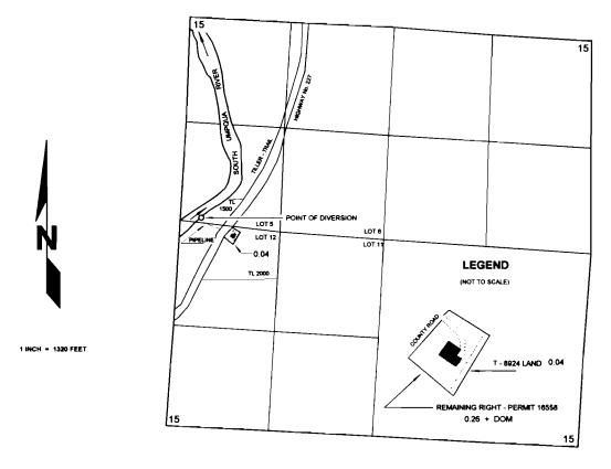
THE POINT OF DIVERSION IS LOCATED 45 FEET NORTH AND 265 FEET EAST FROM THE WEST QUARTER CORNER OF SECTION 15; BEING WITHIN THE SW%, NW% (LOT 5) OF SECTION 15, TOWNSHIP 30 SOUTH, RANGE 4 WEST, W.M.; DOUGLAS COUNTY.
