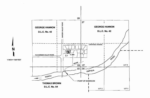
THE POINT OF DIVERSION IS LOCATED 250 FEET SOUTH AND 890 FEET WEST FROM THE NORTHEAST CORNER OF SECTION 33; BEING WITHIN THE NE½ NE½ OF SECTION 33, AS PROJECTED WITHIN D.L.C. 42, TOWNSHIP 26 SOUTH, RANGE 6 WEST, W.M.; DOUGLAS COUNTY.
