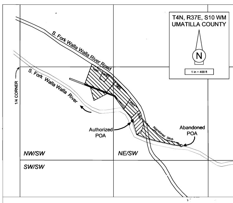
POD is jet pump intake in the South Fork Walla Walla River, located 760 feet South and 1590 feet East from the West Quarter-Corner of Section 10.
