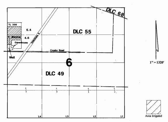
Well is located 670'N & 118'E from the W1/4 corner of Section 6.
