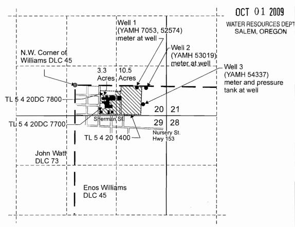
Well 1 (YAMH 7053) is located 65 feet south and 1640 feet east from the NW corner of Williams DLC 45. Well 2 (YAMH 53019) is located 80 feet south and 1870 feet east from the NW corner of Williams DLC 45 Well 3 (YAMH 54337) is located 510 feet south and 1805 feet east of the NW corner of Williams DLC 45
