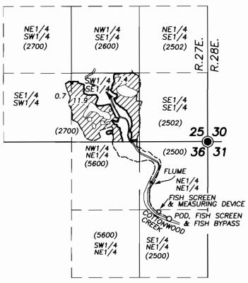
POD IS 1495 FT. SOUTH & 745 FT. WEST OF NE COR. SEC. 36 FISH SCREEN AND MEASURING DEVICE ARE 240 FT. NW'LY OF POD
