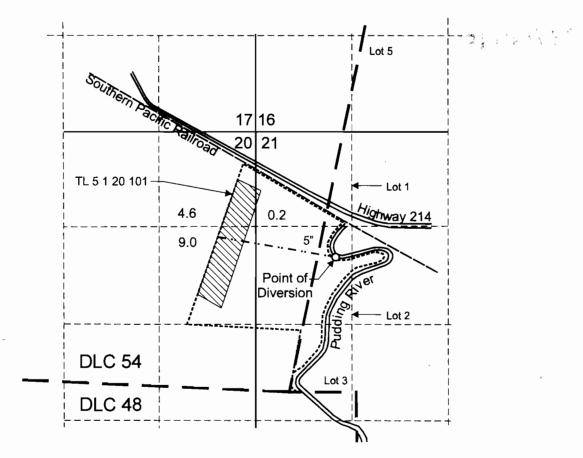
Point of Diversion is located 1,860 feet north and 640 feet east from the SE corner, DLC 54.
