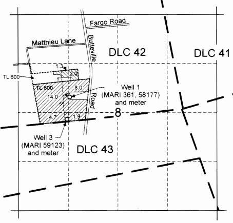
Well 1 (MARI 361, 58117) is located 330 feet north and 3,019.5 feet west from the SE corner of DLC 42. Well 3 (MARI 59123) is located 280 feet south and 3,090 feet west from the SE corner of DLC 42.
