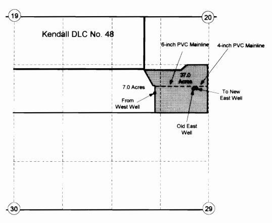
Old East Well was located 530 feet south and 1,340 feet east of the southeast corner of the Kendall DLC No. 48. New East Well is located 520 feet south and 1,400 feet east of the southeast corner of the Kendall DLC No. 48. Existing West Well is located 660 feet south and 280 feet east of the southeast corner of the Kendall DLC No. 48.
