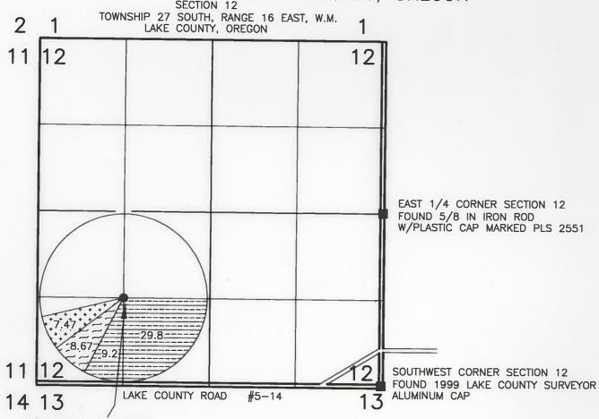
WELL NO. 1 NEW POINT OF APPROPRIATION LOCATED 1369.1' NORTH AND 3971.6' WEST FROM THE SOUTHEAST CORNER OF SECTION 12. AND SITUATED IN THE NW1/4 OF THE SW1/4
