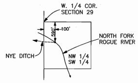
NYE DITCH DIVERSION POINT T.32S.,R.3E.,W.M. SCALE 1" = 1320'
