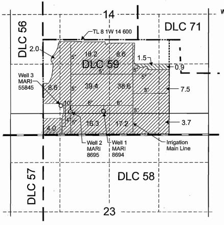
Well 1 (MARI 8694) is located 630 feet north and 1,620 feet east of the southwest corner of T. Fine DLC 59. Well 2 (MARI 8695) is located 620 feet north and 730 feet east of the southwest corner of T. Fine DLC 59. Well 3 (MARI 55845) is located 780 feet north and 480 feet east of the southwest corner of T. Fine DLC 59.
