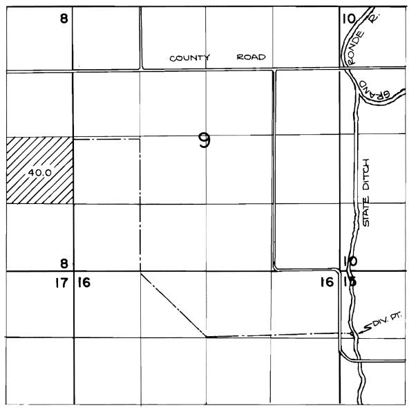
DIVERSION POINT IS LOCATED 1900'S. AND 230'E. FROM THE N.W. CORNER OF SECTION 8 , T.25., R.39E., N.M.
