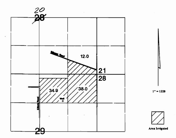
Well is located 1250'S & 1550'W from the NE corner of Section 29.
