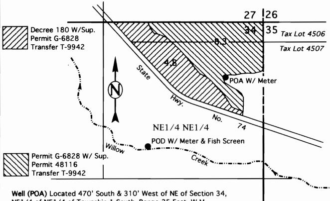
Well (POA) Located 470' South & 310' West of NE of Section 34, NE1/4 of NE1/4 of Township 1 South, Range 25 East, W.M., (Lat. N 45° 26' 32.27837", Lon. W 119° 40' 43.44862") W/ Meter Just 10 Ft. West of Well in 3" Mainline
