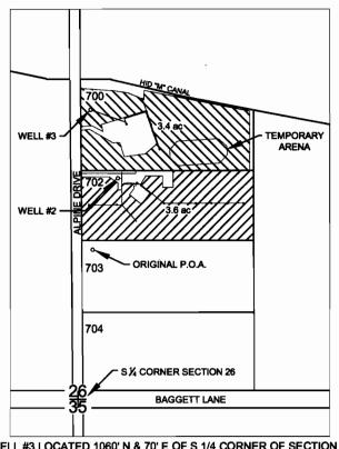
WELL #3 LOCATED 1060' N & 70' E OF S 1/4 CORNER OF SECTION 26. WELL #2 LOCATED 830' N & 180' E OF S 1/4 CORNER OF SECTION 26.
