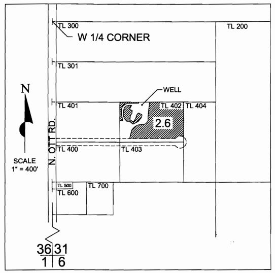
WELL LOCATED 680 FEET SOUTH & 740 FEET EAST FROM THE W1/4 CORNER OF SECTION 31
