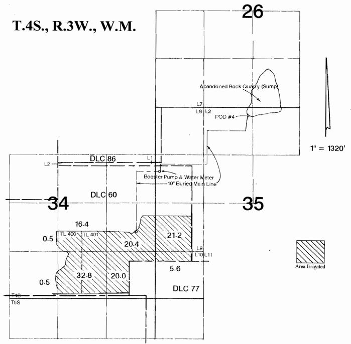
POD #4 is located 240'S & 2620'E from the NW corner of Section 35.
