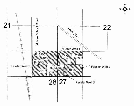
Lichte Well 1: 1040' N & 20' E Fessler Well 1: 630' N 3 1000' W Fessler Well 2: 550' N & 1290' E Fessler Well 3: 20' N & 460' E all from the SW corner Section 22
