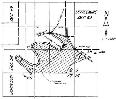
DIV. PTS. LOCATED: ORIGINAL - 100'S AND 675'W. WELL (ADDITIONAL) - 160'N. AND 530'W. BOTH FROM S'LY SW COR. DLC 53
