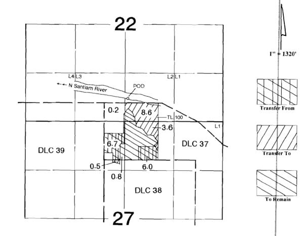
POD is located 120' N & 610' E from the NW corner of DLC 37.
