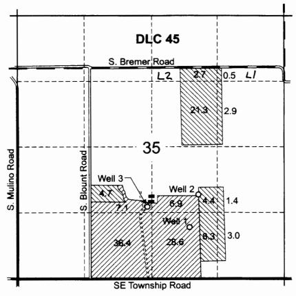
Well 1 (CLAC 12134) is located 1,040 feet north and 1,890 feet west of the southeast corner of Section 35 Well 2 (CLAC 12135) is located 1,700 feet north and 1,700 feet west of the southeast corner of Section 35 Well 3 (CLAC 54906) is located 1,460 feet north and 2,750 feet west of the southeast corner of Section 35
