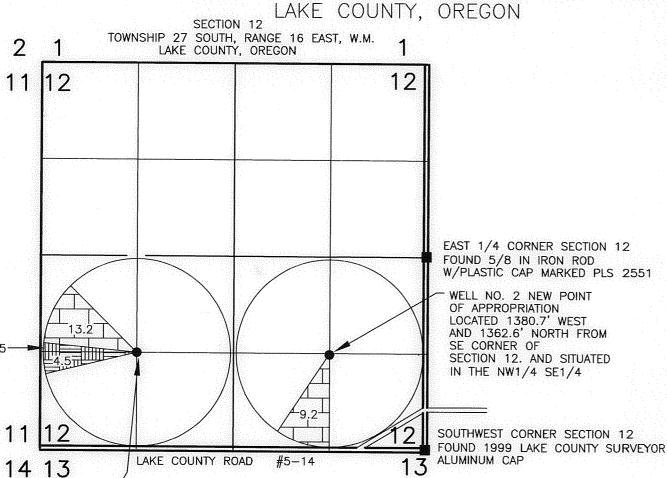
WELL NO. 1 NÉW POINT OF APPROPRIATION LOCATED 1369.1' NORTH AND 3971.6' WEST FROM THE SOUTHEAST CORNER OF SECTION 12. AND SITUATED IN THE NW1/4 OF THE SW1/4
