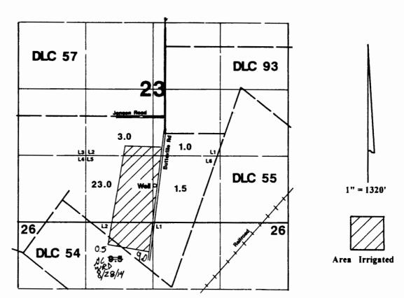
Well is located 740'N & 54'E from the S 1/4 corner of Section 23.
