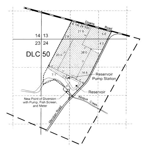
Point of Diversion is located 250 feet north and 1,270 feet east from the W 1/4 corner of Section 24.
