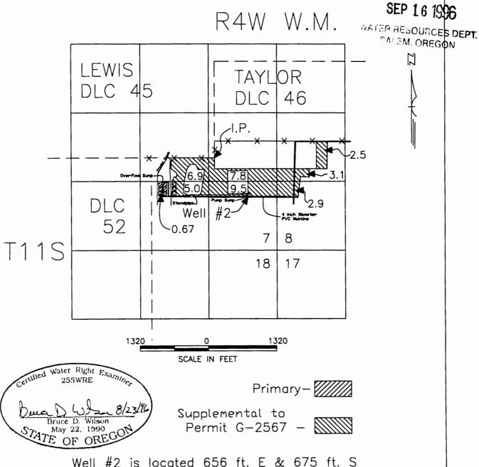
Well #2 is located 656 ft. E & 675 ft. S from the most southerly S.E. corner of Lewis DLC 45 marked with an iron pipe (I.P.).
