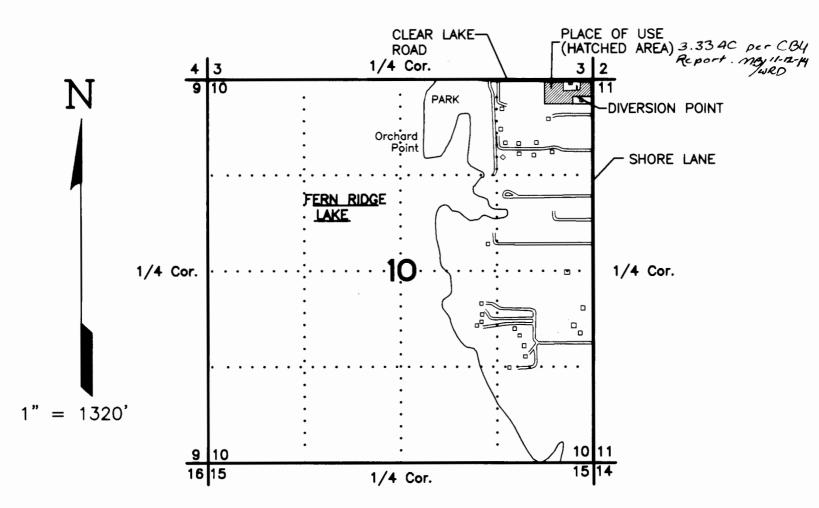
THE DIVERSION POINT IS LOCATED 250' SOUTH AND 200' WEST OF THE N.E. CORNER OF SECTION 10.
