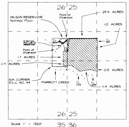
Point of Diversion from Wilson Reservoir is 1166 feet North and 628 feet East of the S.W. Corner D.L.C. No. 44
