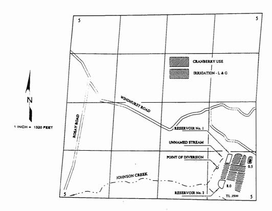
THE POINT OF DIVERSION IS LOCATED 900 FEET NORTH AND 1040 FEET WEST; AND RESERVOIR No. 1 IS LOCATED 1160 FEET NORTH AND 780 FEET WEST; AND RESERVOIR No. 2 IS LOCATED 410 FEET NORTH AND 1000 FEET WEST; ALL FROM THE SOUTHEAST CORNER OF SECTION 5, ALL WITHIN THE SE'/SE'/L OF SECTION 5, TOWNSHIP 29 SOUTH, RANGE 14 WEST, W.M.; COOS COUNTY.
