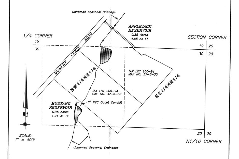
The reservoir locations and configurations shown on this plat are derived from field surveys and survey plats provided by Three Rivers School District as prepared by Tallak D. Maakestad, C.W.R.E. 246. Field inspections were made and locations were checked against aerial photography dated June 9, 1995.
