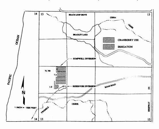
THE SUMPWELL POINT OF DIVERSION IS LOCATED 140 FEET SOUTH AND 890 FEET EAST; AND THE RESERVOIR POINT OF DIVERSION IS LOCATED 970 FEET SOUTH AND 1180 FEET EAST, BOTH FROM THE EAST QUARTER CORNER OF SECTION 13, BEING WITHIN THE NW/SW/4 OF SECTION 13, TOWNSHIP 29 SOUTH, RANGE 15 WEST, W.M.; COOS COUNTY.
