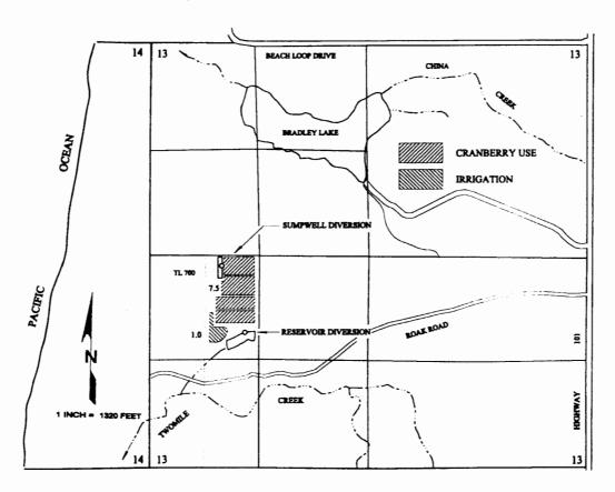
THE SUMPWELL POINT OF DIVERSION IS LOCATED 140 FEET SOUTH AND 890 FEET EAST; AND THE RESERVOIR POINT OF DIVERSION IS LOCATED 970 FEET SOUTH AND 1180 FEET EAST, BOTH FROM THE EAST QUARTER CORNER OF SECTION 13, BEING WITHIN THE NW%SW% OF SECTION 13, TOWNSHIP 29 SOUTH, RANGE 15 WEST, W.M.; COOS COUNTY.
