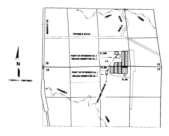
POINT OF DIVERSION No. 1 AT NELSON RESERVOIR No. 1 IS LOCATED 350 FEET SOUTH AND 300 FEET EAST FROM THE NORTH QUARTER CORNER OF SECTION 19, BEING WITHIN THE NWWNEW OF SECTION 19; AND POINT OF DIVERSION No. 2 AT NELSON RESERVOIR No. 2 IS LOCATED 420 FEET NORTH AND 700 FEET EAST FROM THE NORTH QUARTER CORNER OF SECTION 19, BEING WITHIN THE SWYSEW OF SECTION 18; BOTH IN TOWNSHIP 29 SOUTH, RANGE 14 WEST, W.M.; COOS COUNTY.
