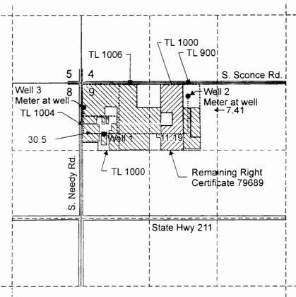
Well 1 (CLAC 2418) is located 1,004 feet south and 440 feet east from the NW corner of Section 9. Well 2 (CLAC 2423) is located 265 feet south and 2,070 feet east from the NW corner of Section 9. Well 3 (CLAC 57441) is located 480 feet south and 50 feet east from the NW corner of Section 9.
