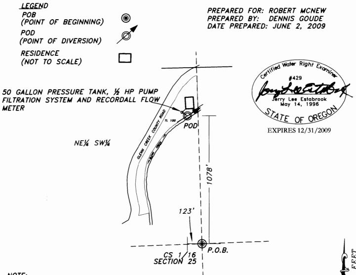
NOTE: THE POINT OF DIVERSION IS AN INSTREAM SCREENED FOOT VALVE 123 FEET WEST AND 1078 FEET NORTH FROM THE CS 1/16 OF SECTION 25, TOWNSHIP 24 SOUTH RANGE 11 WEST, W.M.
