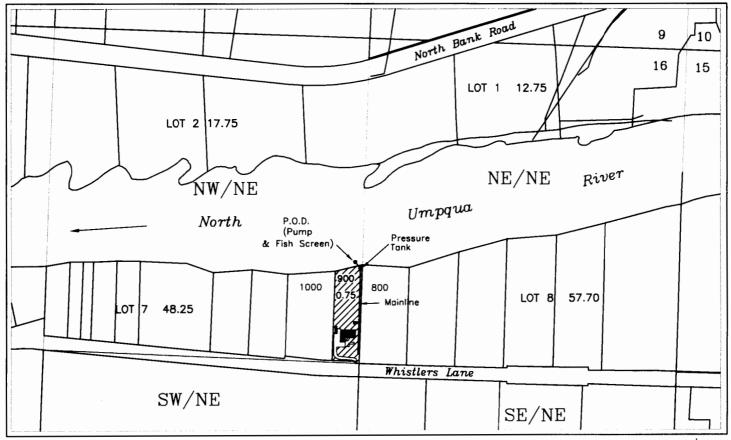
P.O.D. — Pump location — 940 feet south & 1340 feet west from the NE corner section 16
