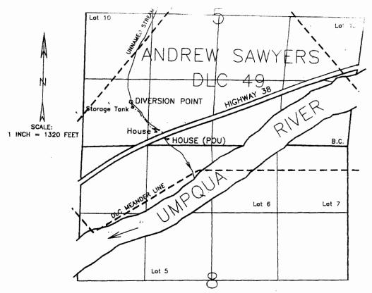
THE DIVERSION POINT IS LOCATED 800 FEET NORTH AND 4300 FEET WEST FROM THE SOUTHEAST CORNER OF SECTION 5.
