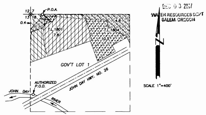
AUTHORIZED DIV. PT. IS 1090' S. AND 30' E. OF THE NW COR. SEC. 18 - C-48346 & C-53320 POINT OF APPROPRIATION IS 2' S. AND 160' E. OF THE NW COR. SEC. 18 INLINE FLOW METER IS S50°E 125 FT. FROM WELL
