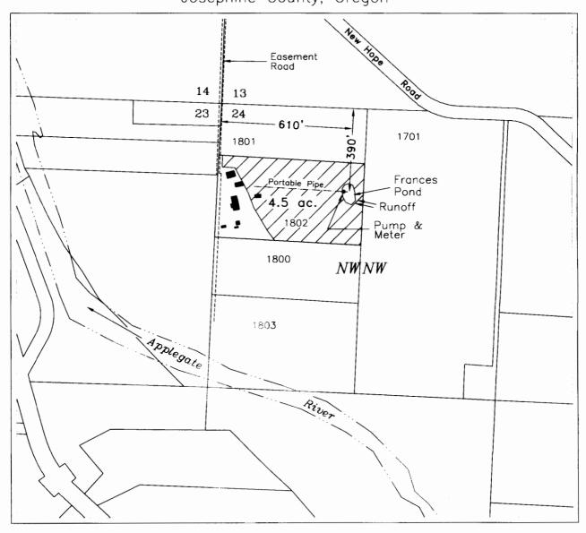
POINT OF DIVERSION — (Center of Pond) NW/NW, 390 feet south & 610 feet east from the NW Corner section 24, T.37S, R.6W, W.M.
