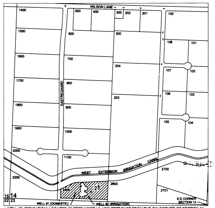
WELL #2 (IRRIGATION) LOCATED 60 FEET NORTH & 1060 FEET EAST FROM THE SW CORNER OF SECTION 14 WELL #1 (DOMESTIC) LOCATED 100 FEET NORTH & 860 FEET EAST FROM THE SW CORNER OF SECTION 14
